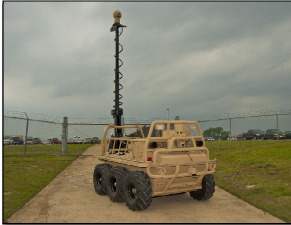
Figure 10: One of many possible Mission Equipment Packages (MEP), RSTA SMSS version for AEWE.
