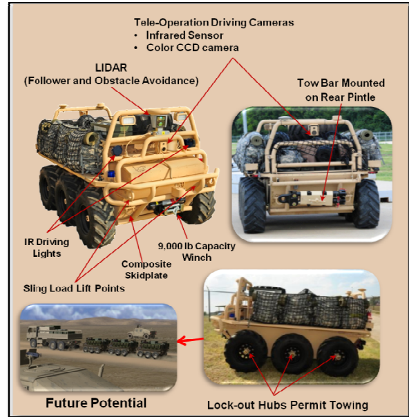
Figure 3: SMSS Block I configuration and features.
