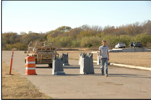
Figure 8: SMSS Following a Person Through Closely Spaced Obstacles. The Person Walked Between Barrels While the SMSS Went Around.
